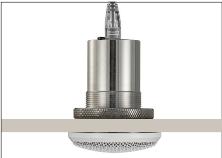
FIGURE 2 Remove the knurled ring from the module, insert the module through the hole and reattach the knurled ring. Connect RJ45 cable to the M70 module.
