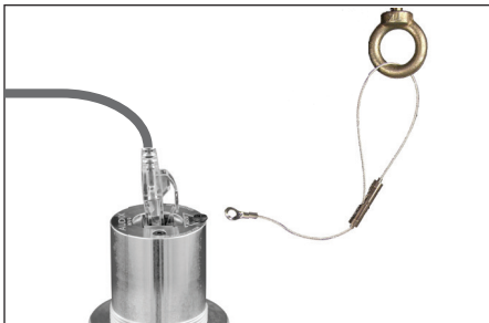
FIGURE 3 For seismic cable installation, wrap the cable through beam, eyebolt or hanger and cable stay barrel (see figure 4). Remove M70WD placement screw and place eyelet over hole and tighten screw.
